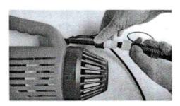
3. Connect and tighten the inlet pipe to the air gun and he outlet pipe of the sprayer
