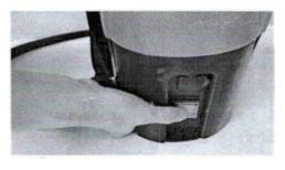
3. Turn on the power switch of the sprayer.
